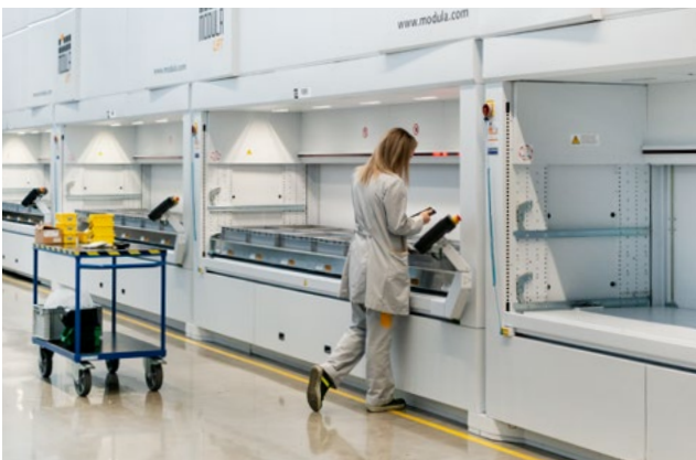
Automated vertical storage system
