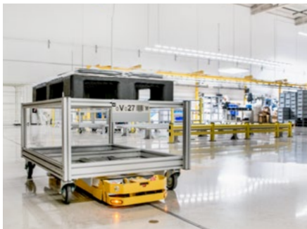
Automated guided vehicle for flexible internal logistics
